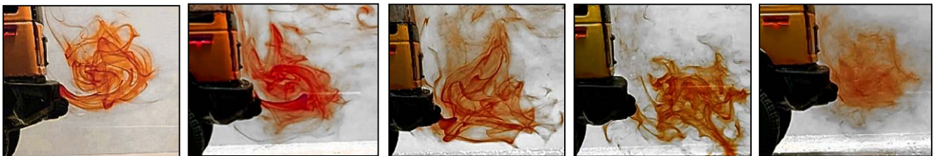
Figure 9: Flow visualization of the bottom vortex branch at Re_L = 7000 (a), 9700 (b), 13800 (c), 20800 (d), and 27700 (e).
