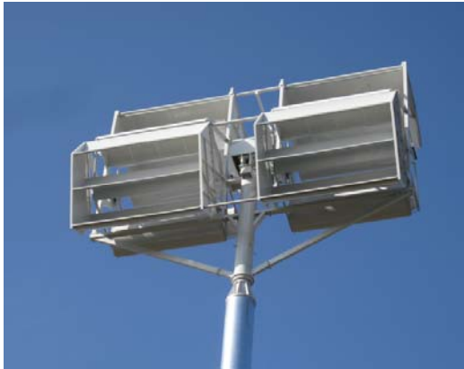
Fig. 7 Photo of 5kW dual-rotor vertical wind turbine at Huber site (Overland Park, Kansas)
