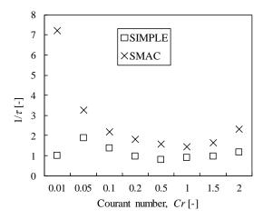
**Figure 6:** Computational speed at t = 1.3 s
