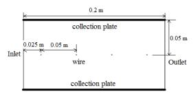
Figure 2: Simulation domain and its dimensions
