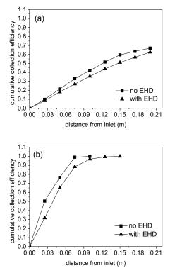
Figure 5: Cumulative collection efficiency for V=40kV and  $d_p$ =1.5  $\mu$ m: (a)  $u_0$ =1.8 m/s; (b)  $u_0$ =0.3 m/s
