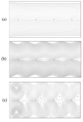
**Figure 3**: Flow streamlines for various N<sub>EHD</sub>: (a) 0; (b) 10.3; (c) 15.6:
