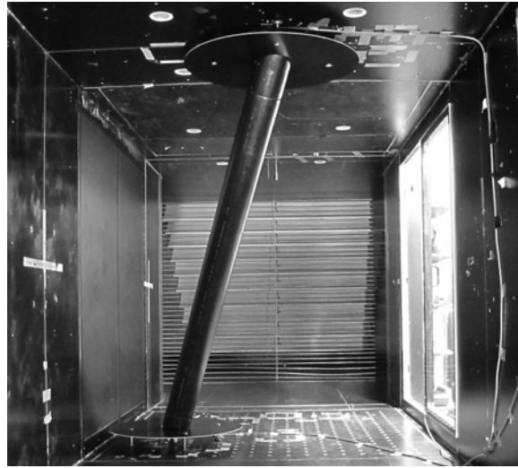
Figure 1. Full-scale, yawed cable model (dry tests).
