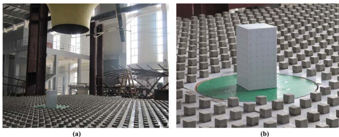
Figure 3 (a) the equipment of the experimental simulation (b) model building dimensions and pressure tap locations
