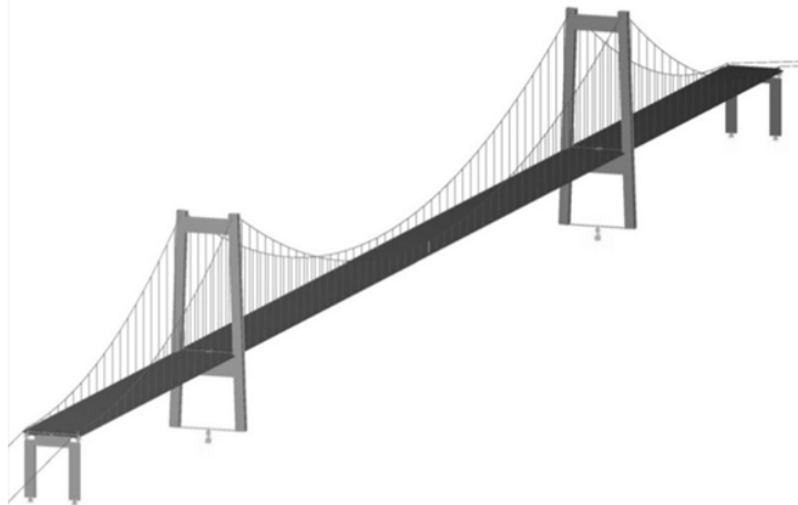
Figure 9. View of full 3D Finite Element bridge model.
