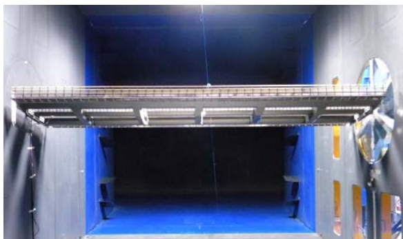
Figure 5. Deck sectional model in wind tunnel (external balance).
