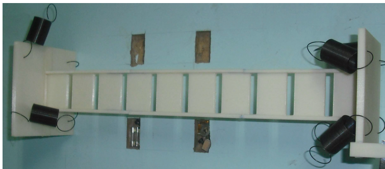
Figure 4. Model with of W/D=4.0 and porosity ratio of 10% ready to be tested
