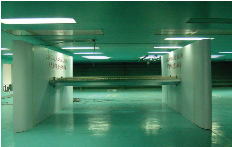
Figure 7 Large-scale sectional model and supporting system
