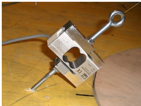
Figure 5. Force transducer for measuring forces in guys.
