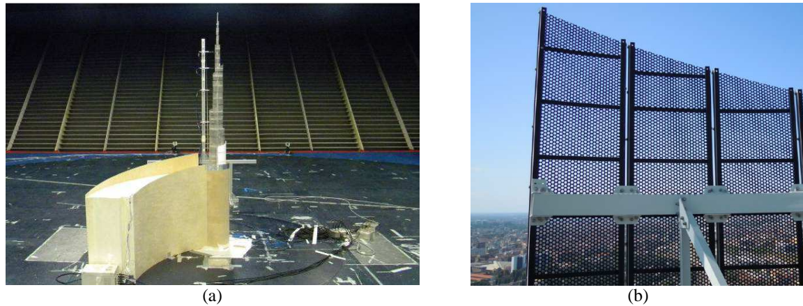
Figure 3. (a) The aeroelastic model in wind tunnel test section. (b) The perforated panels on the real structure.
