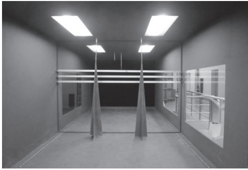
Fig 6. Passive devices for simulation of turbulent wind field of boundary layer.
