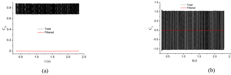
Figure 9 Total and self-excited aerodynamic force time histories on forced vibration cables ( V_r=1050 )
