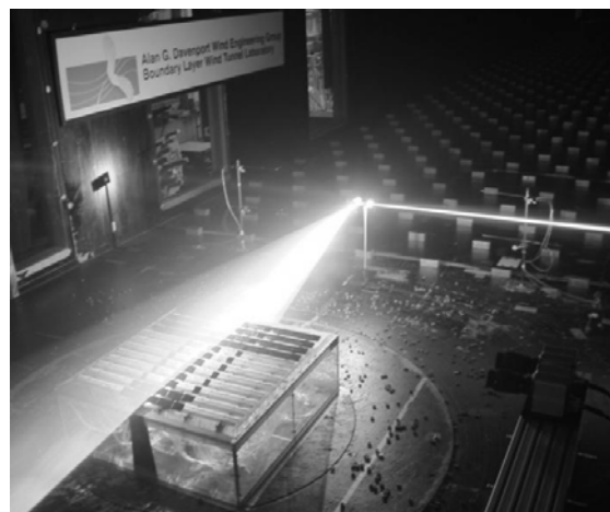
Figure 2. Photograph of experimental setup showing positioning of cameras and laser sheet
