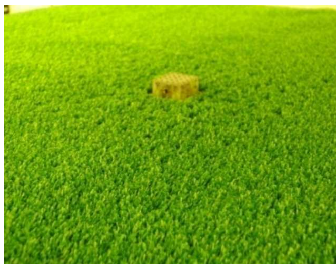
Figure 2. Building model exposed to artificial roughness
