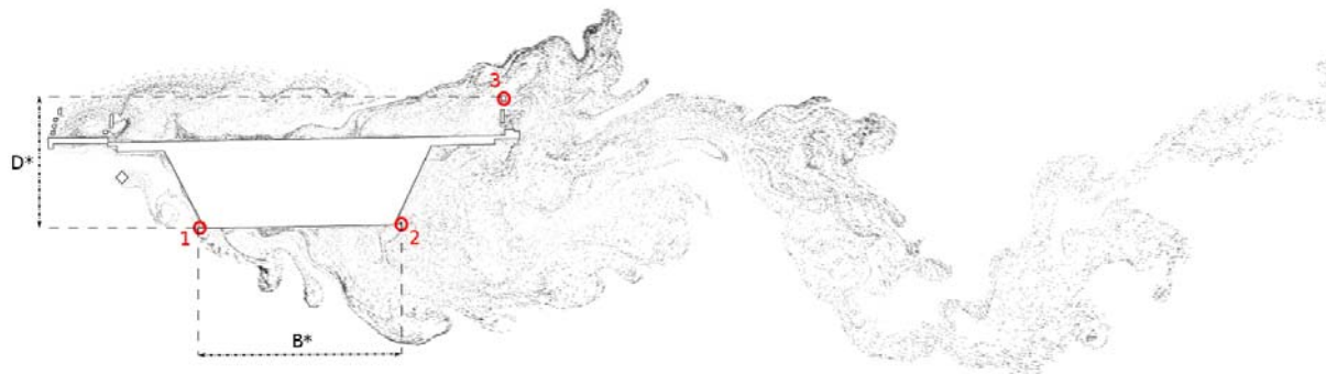
Figure 3. Flow visualization through vortex streaks and effective dimensions of cross-section with bars
