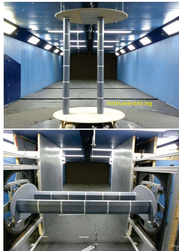
Figure 8: Tower 1:100 sectional model test
