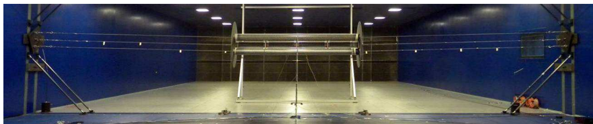
Figure 5. Overall view of the suspended model in the test section for dynamic tests.
