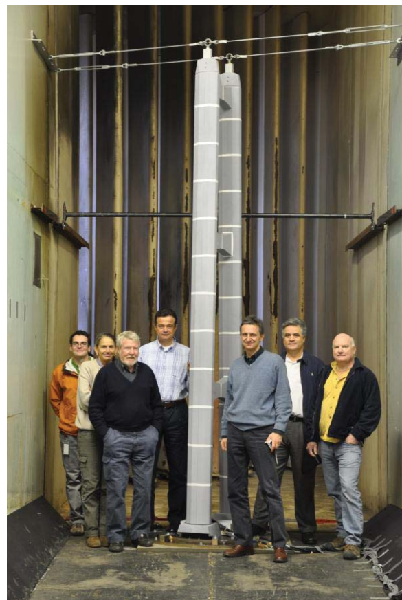
Figure 1: Tower 1:100 aeroelastic model, In-Service configuration.
