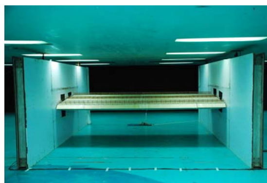
Figure 3. Sectional model in TJ-3 wind tunnel
