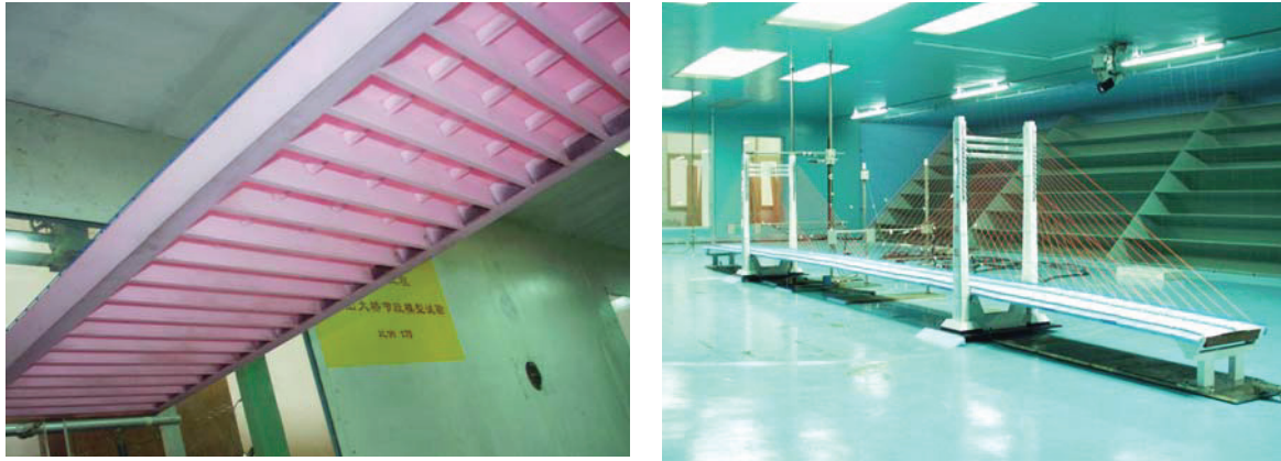
Figure 2 Sectional model and aeroelastic model wind tunnel test for flutter performance
