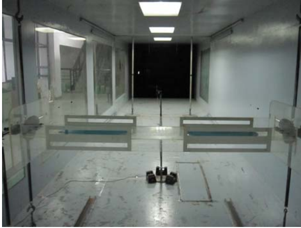
Figure 2 Section model suspended in wind tunnel
