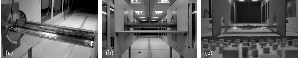
Figure 4. Setups for static tests: isolated deck (a), deck close to plate (b), deck immersed in a boundary layer (c).
