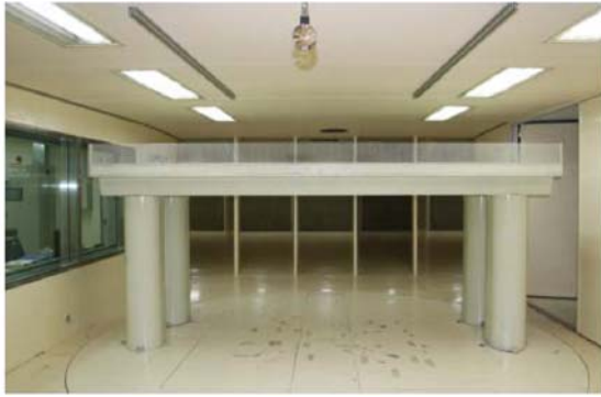
Figure 4. 1/15 scale model of single span bridge in wind tunnel.
