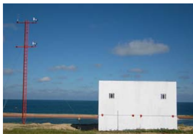
Figure 1. The moveable instrumented building
