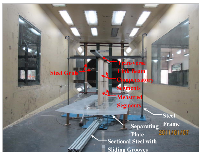
Figure 3 Sectional model in TJ-2 Boundary Layer Wind Tunnel
