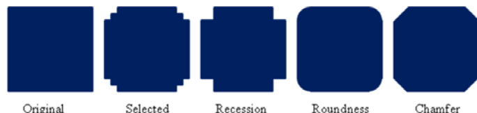
Figure 6. Corner modifications considered in Taipei 101 design
