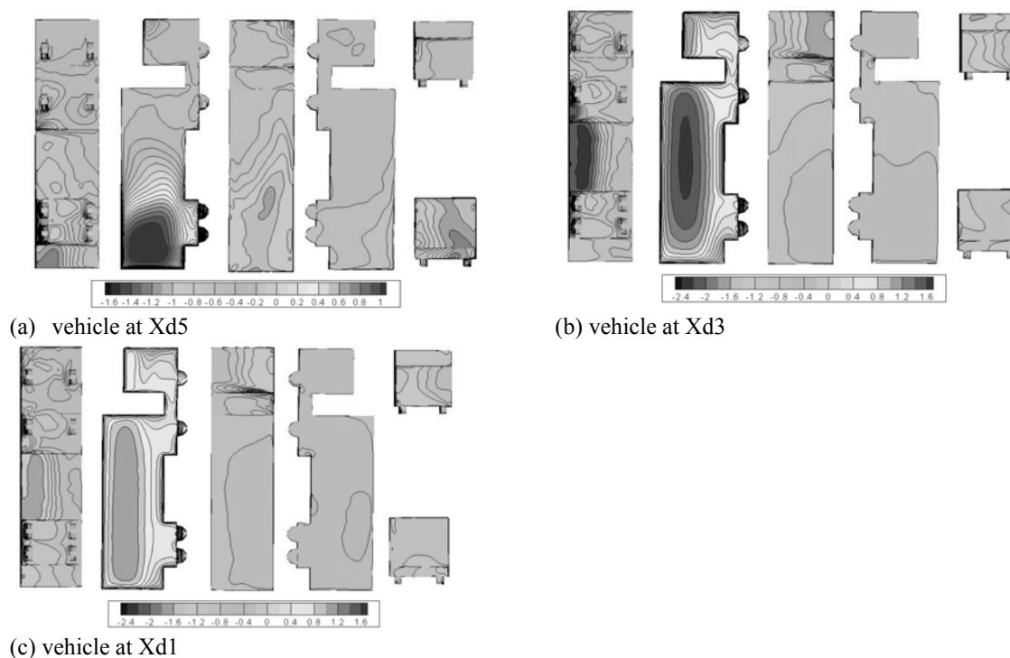
Figure 15. Mean pressure distribution on vehicle (unit: Pa)
