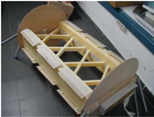
Figure 9. Sectional model of the arch with guide vanes
