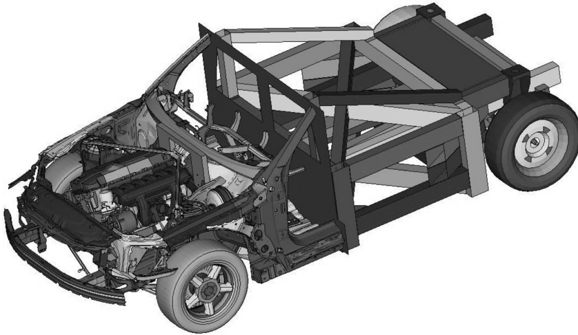
Fig. 4. Simplified FE-model of a car in the concept stage, courtesy of BMW.
