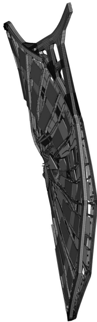
Fig. 3. The buckling mode.
