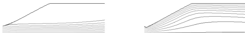
Fig. 3. Streamlines illustrating the flow field in a straight wall (left) and optimum wall (right) diffuser.
