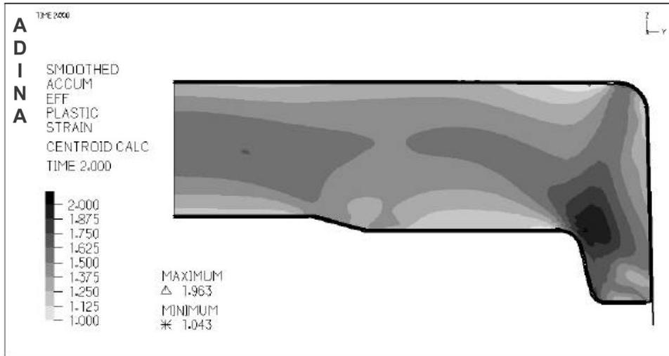
Fig. 4. Plastic strain distribution in the forging without any defects after the second forging cycle.
