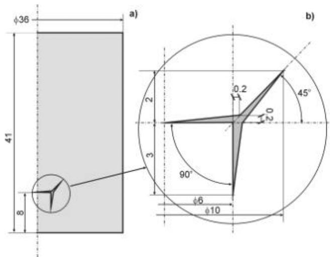
Fig. 2. Defect geometry: (a) a location of the defect in the slug forging, (b) defect dimensions [mm].
