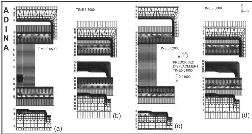
Fig. 1. MES numerical model: (a) the forging with a defect before deformation, (b) the forging with a defect after deformation, (c) the forging with no defect before deformation, (d) the forging with no defect after deformation.
