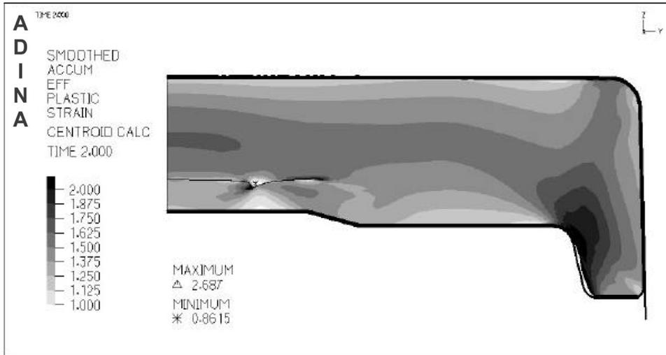
Fig. 3. Plastic strain distribution in the forging with the defect after the second forging cycle.
