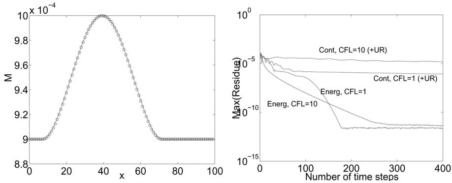
Fig. 1. Subsonic nozzle flow,  $M_t = 0.001$ . (a) Mach number distribution. (b) Convergence plot,  $CFL_u = 1$  and 10. *Energ*: Mach-uniform algorithm with pressure-correction equation based on the energy equation. *Cont*: equivalent algorithm based on the continuity equation (computation with underrelaxation, UR).
