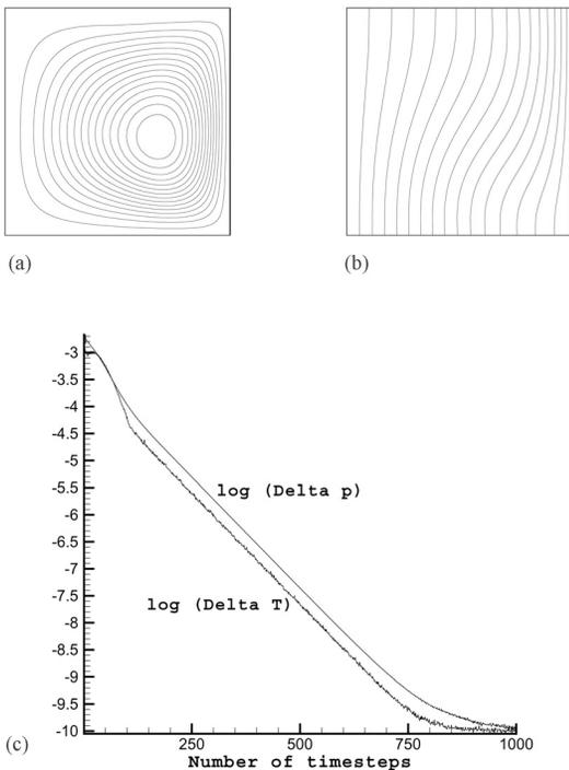
Fig. 3. Thermal driven cavity. (a) Streamline patterns. (b) Temperature contours. (c) Convergence plot.
