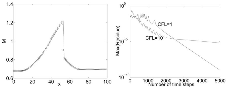
Fig. 2. Transonic nozzle. (a) Mach number distribution. (b) Convergence plot,  $CFL_u = 1$  and 10.
