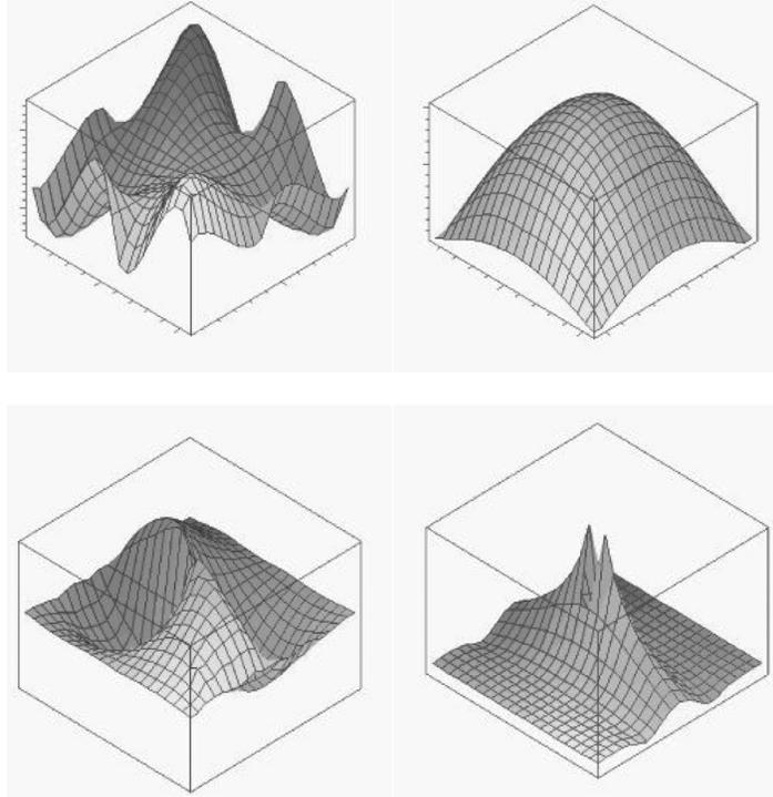
Fig. 1. Perpendicular and parallel displacements of an isotropic (upper row) and anisotropic (lower row) linear elastic medium to a uniform loading (upper row) and a single unit force in the middle of the square (lower row) computed by Fourier BEM [2].
