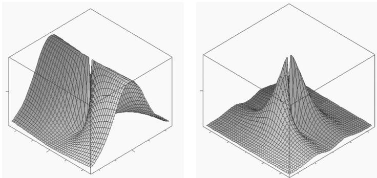
Fig. 3. Integrand of the hyper singular entry in the Fourier space (left) and the same term after accounting for all singular terms of the boundary integral equation [2].
