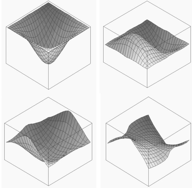
Fig. 2. Isotropic elastic Kirchhoff plate (thin clamped plate) under uniform loading. Upper row: vertical displacements on the left and slope  $\varphi_1$  on the right. Lower row: moment  $m_{11}$  (left) and shear force  $q_1$  (right) computed by Fourier BEM [2].
