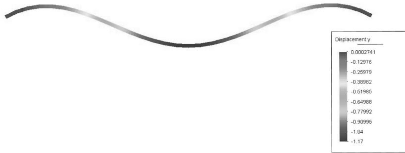
Fig. 4. Vertical displacement at the midpoint ( |\mathbf{f}_{central\ node,y}^{int}| = 4000\text{ N} ).
