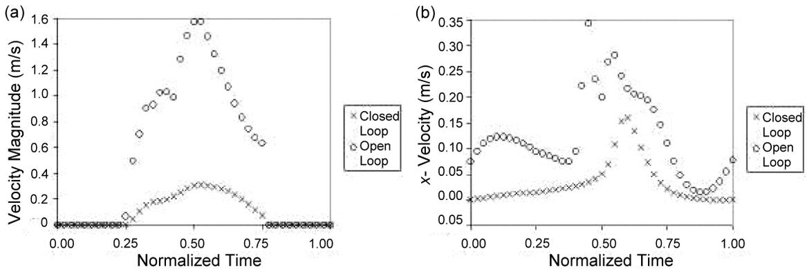
Fig. 3. Comparison of open- and closed-loop results. (a) Velocity magnitudes at the blood chamber inlet; (b)  $x$ -velocities at a point inside the blood chamber.
