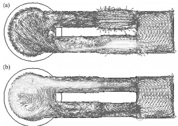
Fig. 2. Velocity vectors at (a) end of ejection and (b) end of filling.
