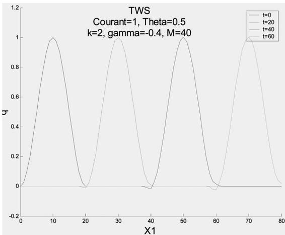
Fig. 6. Unsteady scalar field transport, TWS,  $C = 1.0$ ,  $\theta = 0.5$ ,  $k = 2$ ,  $\gamma = -0.4$ ,  $M = 40$ .
