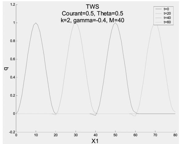
Fig. 4. Unsteady scalar field transport, TWS, C = 0.5,  $\theta = 0.5$ , k = 2,  $\gamma = -0.4$ , M = 40.
