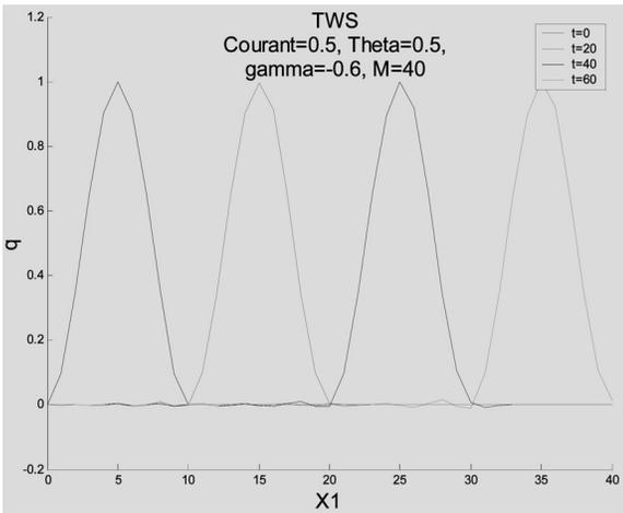
Fig. 2. Unsteady scalar field transport, TWS, C = 0.5,  $\theta = 0.5$ , k = 1,  $\gamma = -0.6$ , M = 40.
