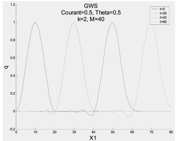
Fig. 3. Unsteady scalar field transport, GWS, C = 0.5,  $\theta = 0.5$ , k = 2, M = 40.
