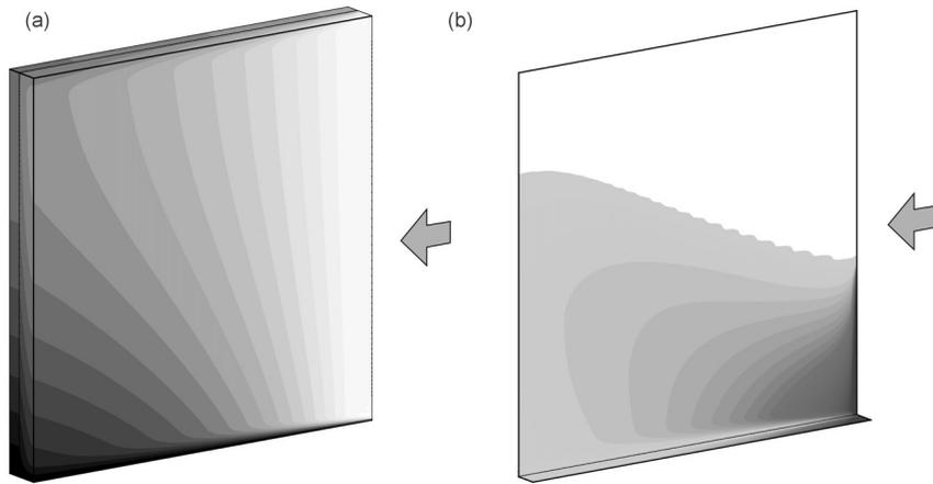
Fig. 2. Moisture condensation on a rectangular plane fin: (a) temperature field and (b) specific mass flow rates of condensing vapour.
