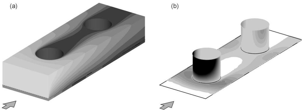
Fig. 3. Moisture condensation in a two-row tube-fin exchanger with an in-line arrangement of tubes: (a) temperature field and (b) specific mass flow rates of condensing vapour.
