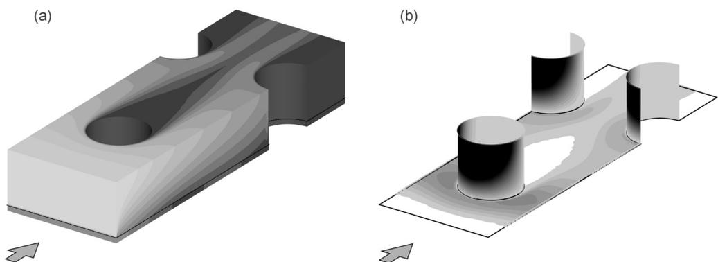
Fig. 4. Moisture condensation in a two-row tube-fin exchanger with a staggered arrangement of tubes: (a) temperature field and (b) specific mass flow rates of condensing vapour.
