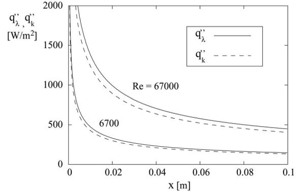
Fig. 1. Sensible and latent heat fluxes on a cold plate in contact with a moving stream of moist air.
