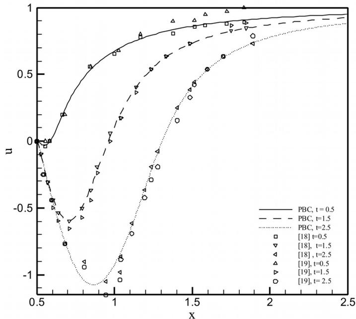
Fig. 3. Horizontal velocity at different locations along the x-axis in the wake at time instants of 0.5, 1.5 and 2.5 for an impulsively started circular cylinder at  $Re = 550$ .
