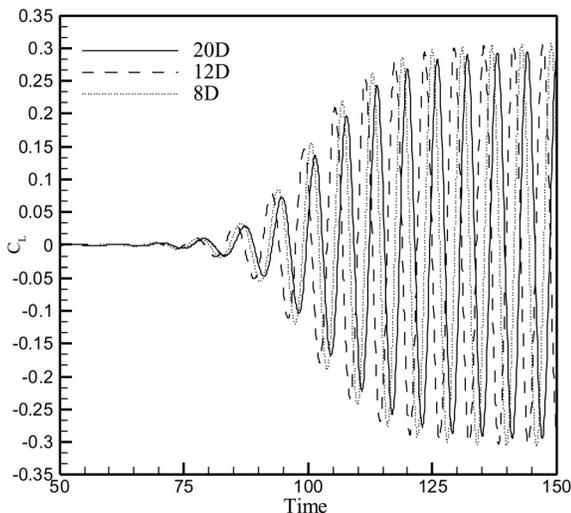
Fig. 1. Variation of coefficient of ( $C_L$ ) at  $Re = 100$  for different boundary placements for flow past a circular cylinder.
