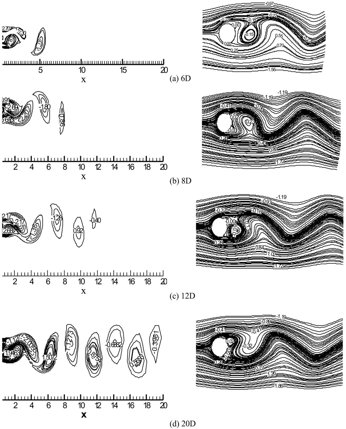
Fig. 2. Instantaneous vorticity and streamline contours for a circular cylinder in the wake for different boundary placements of (a) 6D (b) 8D (c) 12D (d) 20D at  $\tau = 300$  for  $Re = 100$ .
