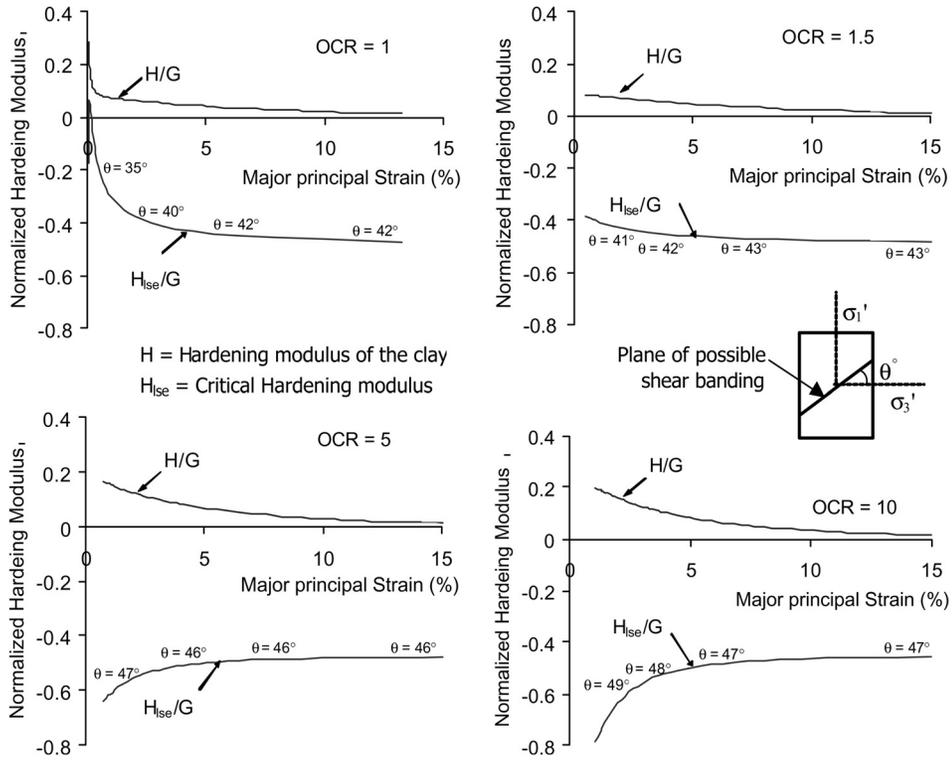
Fig. 2. Critical hardening modulus using the concept of the loss of strong ellipticity, and corresponding inclination of possible shear banding type strain localization.
