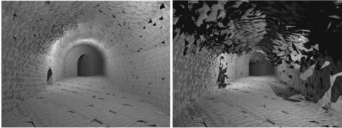
Fig. 6. Snapshots of the largest room at 0ms and 200ms. The simulation predicts that this large room within the facility would completely collapse under the applied loading.
