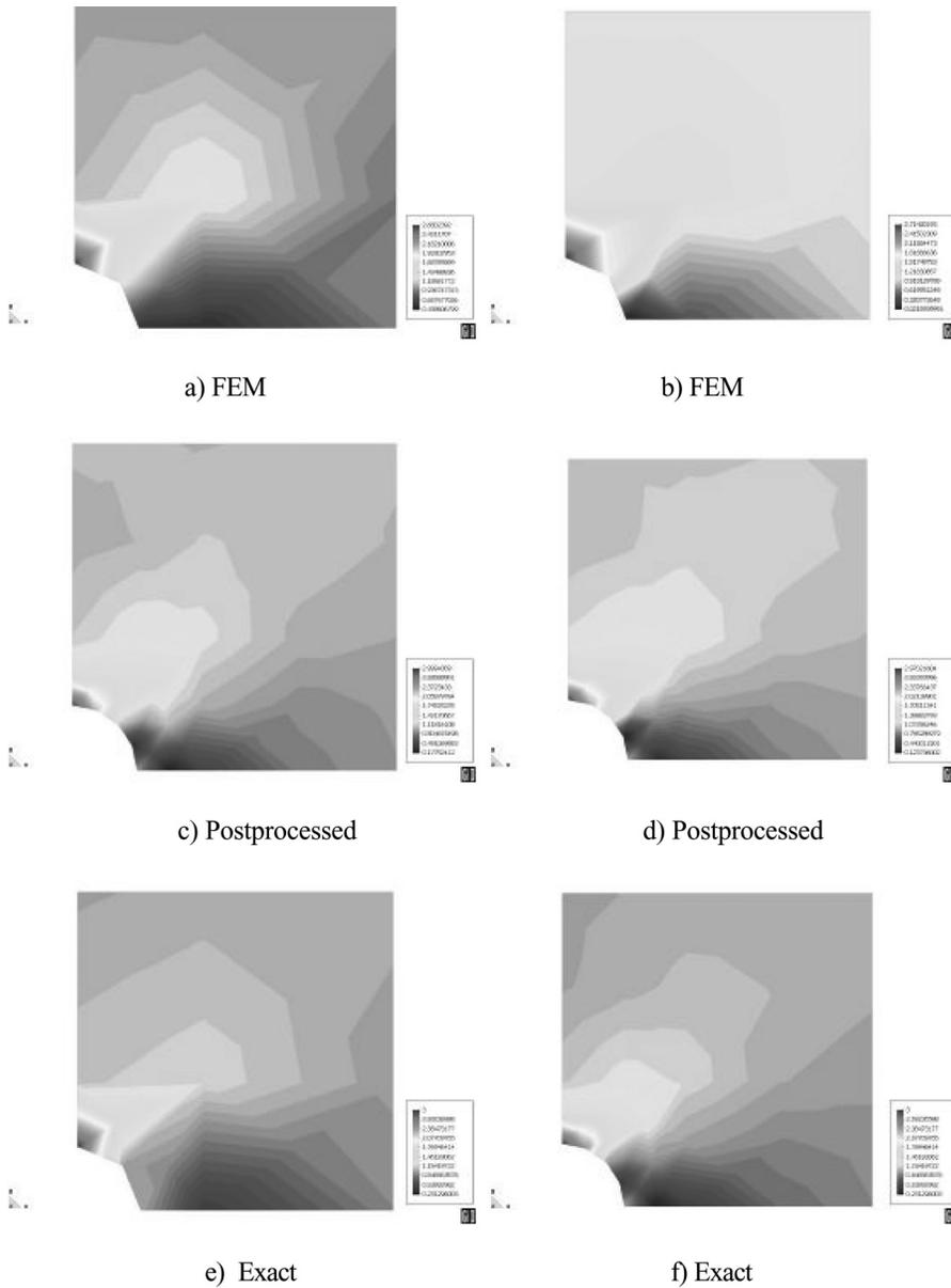
Fig. 3. Von Mises stress fields obtained by the averaging technique in FEM software and by T-interpolation from FEM nodal displacements.
