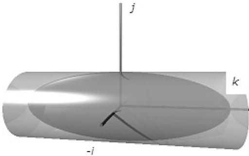
Fig. 1. Rectangular coordinate system for parameterization for the ellipsoid surface, where  $k$  is oriented along the major axis,  $j$  along the semi-minor axis, and  $i$  along the minor axis.
