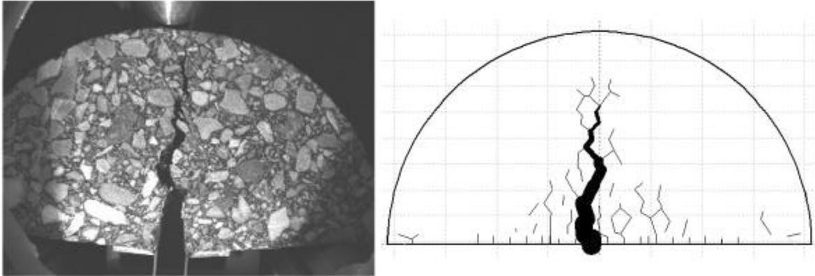
Fig. 3. Comparison between experimental and model crack propagation.
