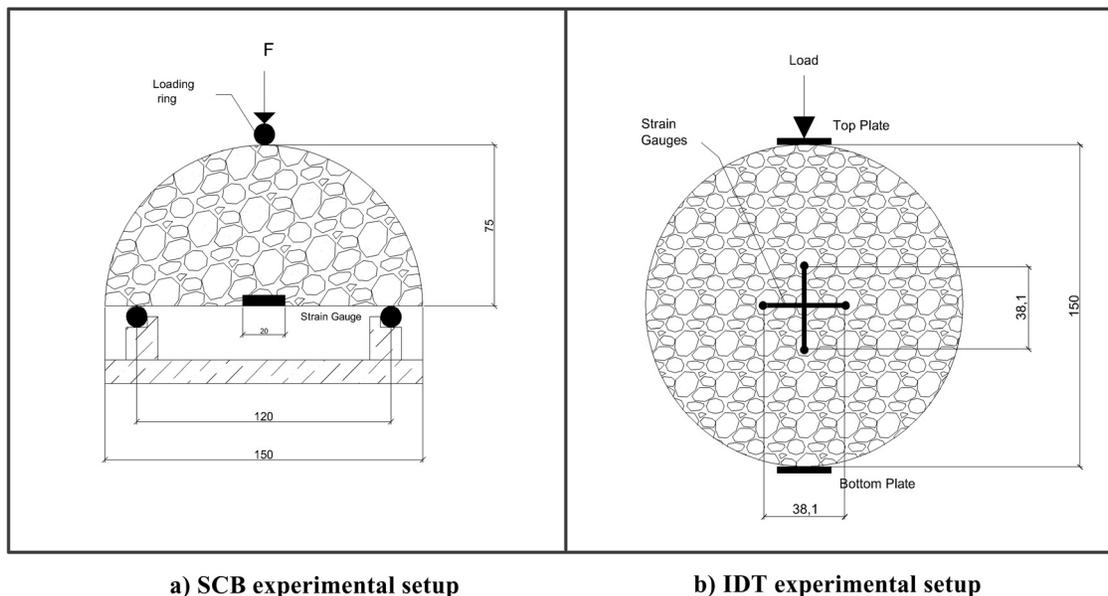
Fig. 1. Experimental setups of both tests. (a) SCB experimental setup; (b) IDT experimental setup.
