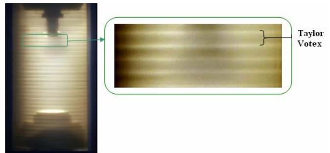
**Figure 3:** Visualization of a state of flow by mean of optical Transmission
