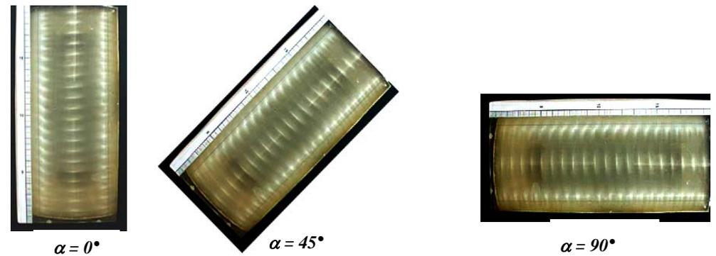
**Figure 8 :** Effect of inclination on the wavy mode  $\Gamma = 40$
