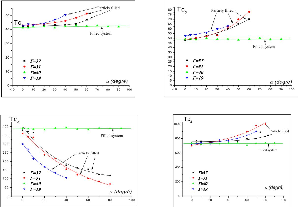
**Figure 5:** Variation of the critical numbers of Taylor  $Tc_1, Tc_2, Tc_3, Tc_4$  versus angle of inclination  $\alpha$  for a given aspect factor  $\Gamma$
