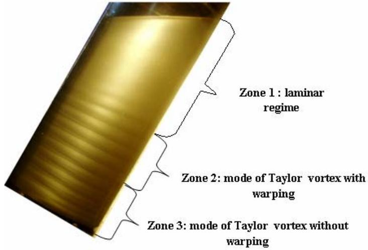
**Figure.6** coexistence of three modes regimes in bending Taylor – Couette Flow
