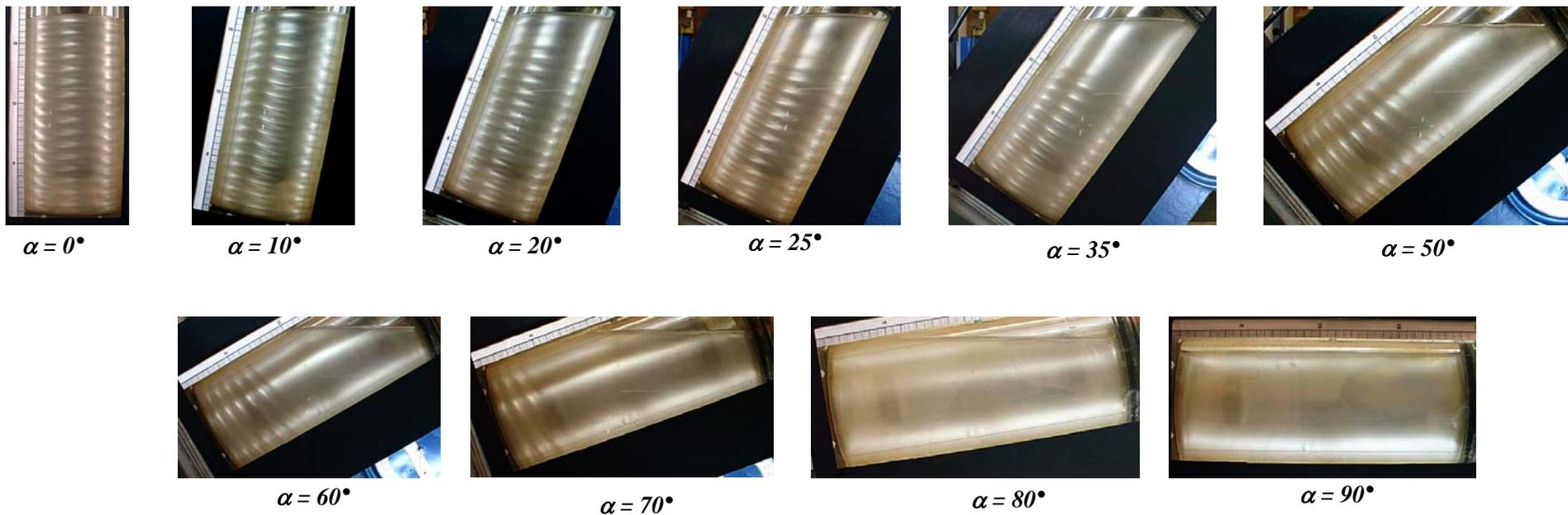
**Figure 10 :** Effect of inclination on the Taylor vortex  $Ta=59,6$  ;  $\Gamma = 37$ .
