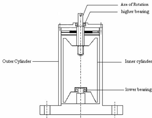
**Figure.1:** apparatus Taylor – Couette flow
