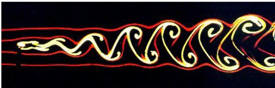
FIGURE 2.2: The Bénard-von Kármán vortex street behind a circular cylinder at  $Re = 65$  (taken from Provansal *et al.* (2004)).
