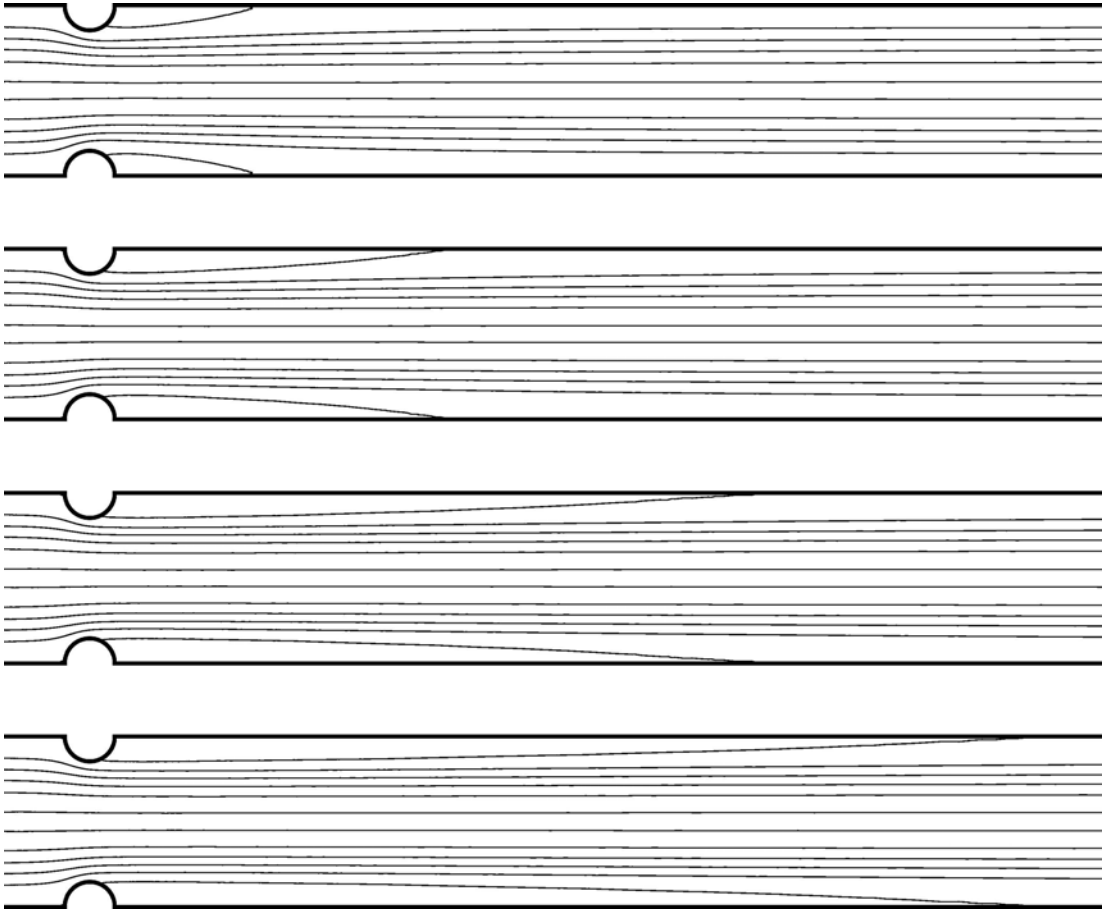
FIGURE 5.2: Streamlines at b = 0.50 and Re = 200, 500, 1000 and 1500 . The terminating streamline indicates the recirculation length.
