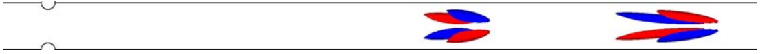
FIGURE 6.13: Two positive and negative contours of the streamwise vorticity of the perturbation mode ( m = 1 ) for b = 0.50 , Re = 500 , A = 0.75 and T = 2.5 ( \alpha = 17.72 ).
