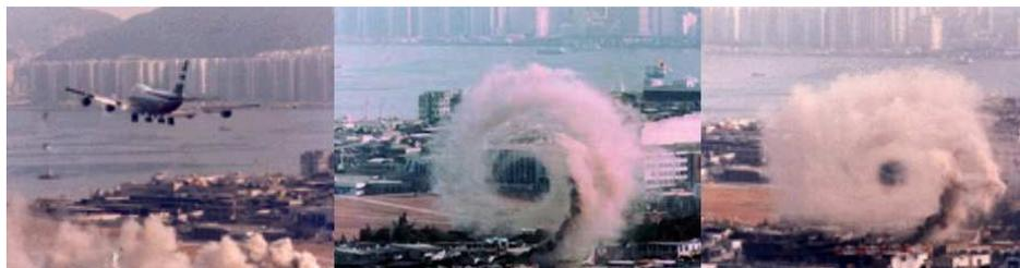
Figure 1.3: One of a pair of strong wing-tip vortices observed in chimney smoke after a landing aircraft passes. Source unknown.
