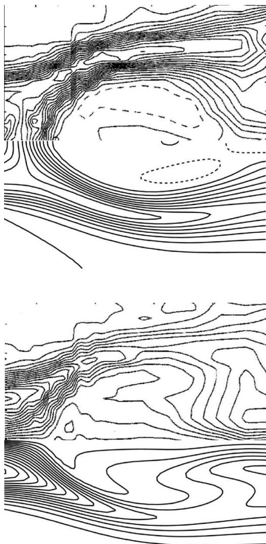
Figure 3.12: Axial (above) and azimuthal (below) velocity contours as measured by Billant *et al.* (1998) at  $Re = 687$ ,  $S = 1.4$  (upper half), and compared to contours from simulations at  $Re = 400$ ,  $S = 1.4$  (lower half). The flow direction is left to right and the dashed lines represent contours of negative velocity. The contours of Billant *et al.* are time averaged, whereas the contours of the simulations are instantaneous.
