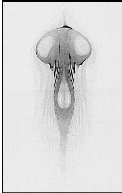
Figure 1.7: Fluorescein dye visualisations of a diametrical plane through a closed cylinder flow displaying dual recirculation bubbles. Reproduced from Sotiropoulos *et al.* (2002).
