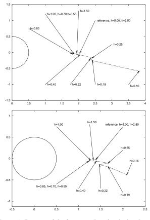
Figure 4: Position of the formation length calculated using the standard deviation in the vertical velocity (top) and vorticity (bottom), for a Froude number of 0.20.
