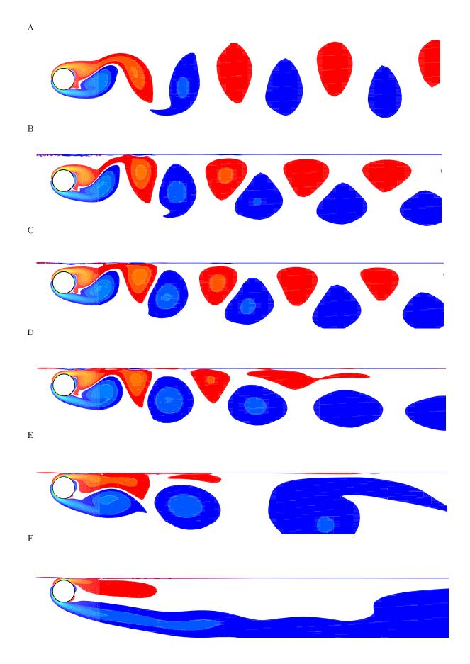
Figure 5: Vortex street plots for: (A) the reference cylinder, (B) gap ratio 0.70 and Froude number 0.20, (C) gap ratio 0.40 and Froude number 0.20, (D) gap ratio 0.25 and Froude number 0.20, (E) gap ratio 0.16 and Froude number 0.20, (F) gap ratio 0.10 and Froude number 0.20
