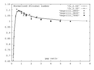
Figure 2: Variation of Strouhal number (normalized with respect to Strouhal number of the reference cylinder i.e.  $\frac{St}{St_0}$ ) with submergence depth, for both the Fr = 0.00 and Fr = 0.20 cases.
