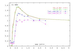
Figure 3: Plot showing the variation of RMS lift coefficient with gap ratio for the free slip (Froude number 0.00) and Froude number 0.20 cases. Also plotted are the results of Lei *et al.* (1999) (for their boundary layers 1 and 2).
