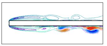
Figure 2 – Spatial structure of dominant instability mode, from Floquet stability analysis. Red and blue indicate +/– spanwise perturbation vorticity, from -0.2 to 0.2; line contours are of spanwise vorticity, indicating positions of von Karman vortices.
