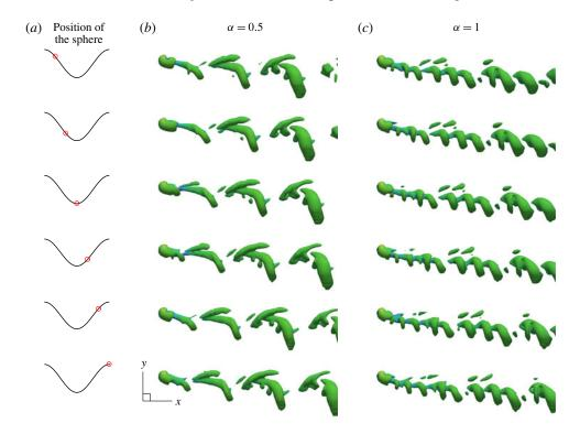
FIGURE 18. (Colour online) Evolution of the wake structures for one cycle of the sphere oscillation in the synchronisation regimes (at  $U^* = 6$ ) for the rotation rates  $\alpha = 0.5$  and 1. The first column displays the position of the sphere by a red 'bullseye' on a cosine wave for one period, while the second and third columns show the instantaneous wake structures observed at each of these positions of the sphere for  $\alpha = 0.5$  and 1 respectively.
