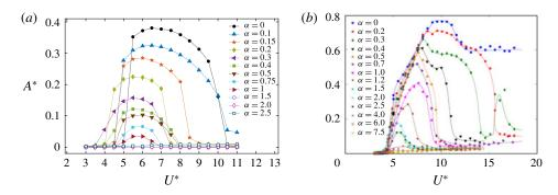
FIGURE 11. (Colour online) The variation sphere response amplitude with reduced velocity at each rotation rate: (a) present results of this numerical study at Re = 300, (b) results of the experimental study of Sareen *et al.* (2018) over the Reynolds number range, Re = 5000-30000.
