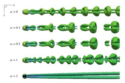
FIGURE 19. (Colour online) Instantaneous wake structures in the xz plane for a transversely rotating sphere at  $U^* = 6$  for the rotation rates  $\alpha = 0$ , 0.3, 0.5, 1 and 2.
