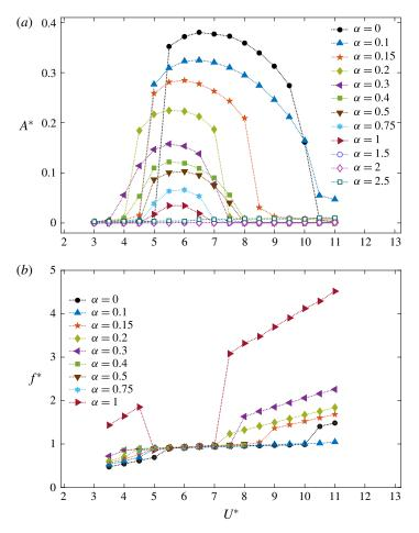
FIGURE 7. (Colour online) The sphere response: (a) the variation of the maximum oscillation amplitude,  $A^*$ , with the reduced velocity,  $U^*$ , at each rotation rate; and (b) the frequency ratio  $f^* = f/f_n$  for rotation rates and reduced velocities at which the sphere showed a vibrational response.
