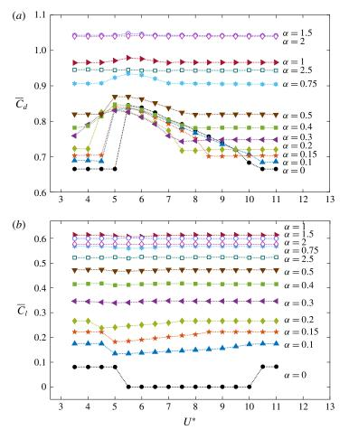
FIGURE 12. (Colour online) Variation of the time-mean (a) drag force coefficient,  $\overline{C}_d$ , and (b) lift force coefficient in the y direction,  $\overline{C}_{ly}$ , with the reduced velocity,  $U^*$ , at each rotation rate.
