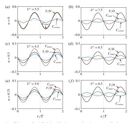
FIGURE 14. (Colour online) Relationship between the time-mean displacement of the sphere, Y/D, the total force in the y direction,  $C_{total}$ , and the vortex force in the y direction,  $C_{vortex}$ , at  $\alpha = 0$ , 0.3 and 0.75: (*a*,*c*,*e*) at mode I, and (*b*,*d*,*f*) at mode II.
