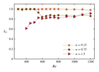
FIGURE 22. (Colour online) Variation of the periodicity of sphere response,  $\lambda_A$ , with Reynolds number at  $\alpha = 0.15$ , 0.75 and 1.5 for  $U^* = 6$ .
