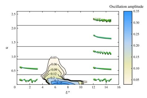
FIGURE 20. (Colour online) Contour plot of the sphere oscillation amplitude,  $A^*$ , as a function of the reduced velocity,  $U^*$ , and rotation rate,  $\alpha$ . The non-synchronisation regime is divided into five regimes according to wake structures.
