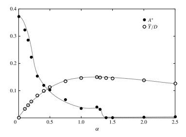
FIGURE 8. Variation of the oscillation amplitude,  $A^*$ , and the time-mean position,  $\overline{Y}/D$ , of the sphere with the rotation rate,  $\alpha$ , at the reduced velocity  $U^* = 6$ .
