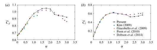
FIGURE 3. (Colour online) Comparison with other numerical studies of computed time-mean drag coefficient,  $\overline{C}_d$ , and time-mean lift coefficient,  $\overline{C}_l$ , for flow past a rigidly mounted and transversely rotating sphere at Re = 300 for  $0 \le \alpha \le 3$ .
