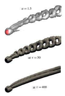
FIGURE 5. (Colour online) Comparison of wake structures of a rigidly mounted and transversely rotating sphere for  $\alpha = 1.5$  with Dobson *et al.* (2014) (the dark structure). The light structures are the results of the present study.
