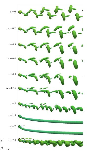
FIGURE 16. (Colour online) Instantaneous wake structures of vortex-induced vibration of a transversely rotating sphere at reduced velocity  $U^* = 6$  at each rotation rate. The sphere showed synchronised vibrations up to  $\alpha = 1$ , and all the synchronisation regimes contained  $U^* = 6$ . Therefore, the wake structures given for  $0 \le \alpha \le 1$  are those in the synchronisation regimes at those rotation rates. The Reynolds number of the flow is Re = 300.
