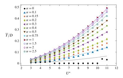
FIGURE 6. (Colour online) Variation of the time-mean position of the sphere,  $\overline{Y}/D$ , with the reduced velocity,  $U^*$ , at each rotation rate: the dotted lines represent the estimated time-mean position of the sphere according to the time-mean lift force,  $\overline{C}_l$ , calculated for a rigidly mounted sphere at each rotation rate ( $\overline{Y}/D = 3\overline{C}_l U^{*2}/(16m^*\pi^2)$ ).
