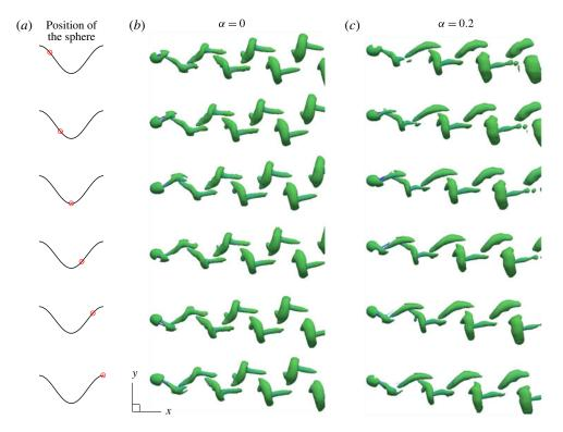
FIGURE 17. (Colour online) Evolution of wake structures for one cycle of sphere oscillation in the synchronisation regimes (at  $U^* = 6$ ) for the rotation rates  $\alpha = 0$  and 0.2. The first column displays the position of the sphere by a red 'bullseye' on a cosine wave for one period, while the second and third columns show the instantaneous wake structures observed at each of these positions of the sphere for  $\alpha = 0$  and 0.2, respectively.
