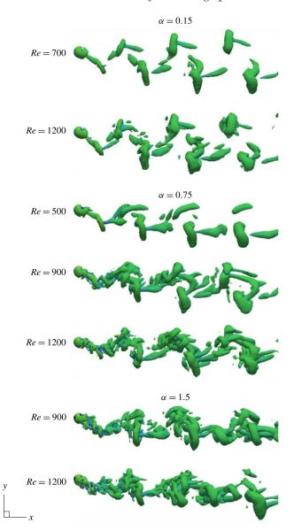
FIGURE 24. (Colour online) Effect of Reynolds number on the wake structures (depicted with Q = 0.01) at the rotation rates  $\alpha = 0.15$ , 0.75 and 1.5. The reduced velocity of the flow is  $U^* = 6$  for each case.
