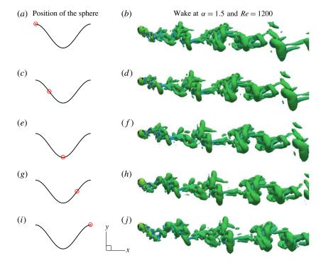
FIGURE 25. (Colour online) Evolution of the wake at  $\alpha = 1.5$ , Re = 1200 and  $U^* = 6$  for a cycle of sphere vibration. The left column shows the sphere position in the cycle with a red 'bullseye' on a cosine wave and the right column shows the wake structures observed at corresponding sphere positions.
