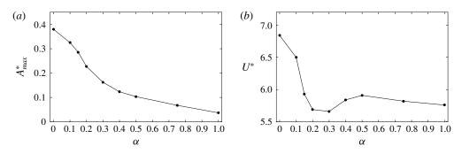
FIGURE 9. Variations of (a) the maximum oscillation amplitude of the sphere,  $A_{max}^*$ , and (b) the reduced velocity at which the sphere showed a maximum oscillation amplitude with the rotation rate,  $\alpha$ .
